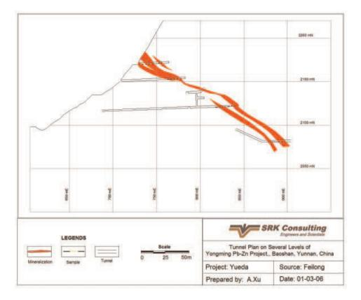
Figure 8 – Cross-Section through V1 Orebody
