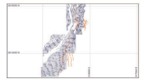
Figure 7 – Outcrop Sketch of the Geology and Location of the Main Ore Bodies
